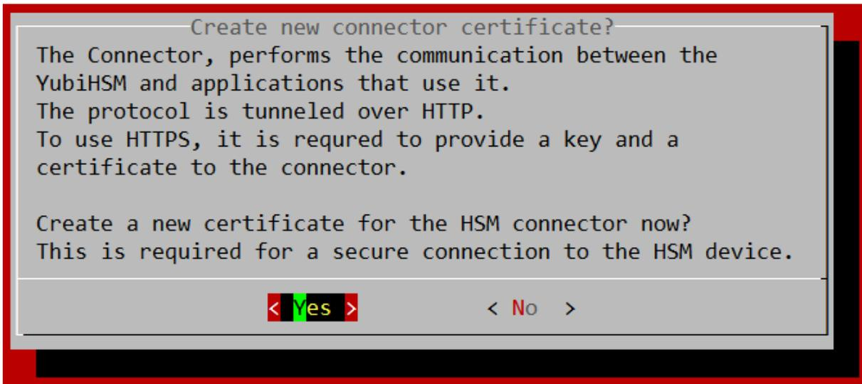
This certificate is not stored on the YubiHSM and is only required for a secure connection from the PKI server to the HSA. (It is used for the nginx HTTPS proxy between the Windows CNG Key Storage Provider and the YubiHSM connector.)
