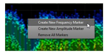
Chanalyzer Lab will build a table on the right-hand side where it will measure the current average and max for each frequency. These values are dependent on the time span selected.
