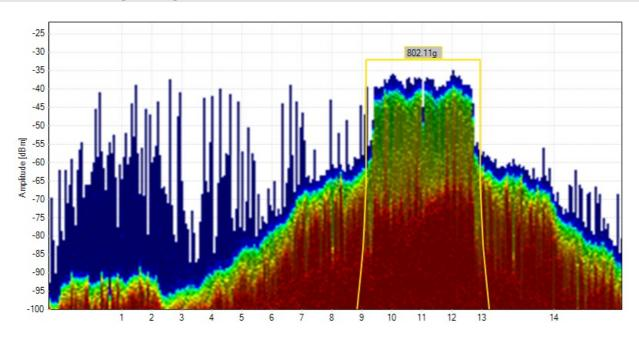
This shape is a **flat table-top shape** with shoulders on either side, which is the signature of an **802.11g** or **802.11n** network. This means that the network is running at faster data rates such as 12, 24, 54 mbps, and beyond.
