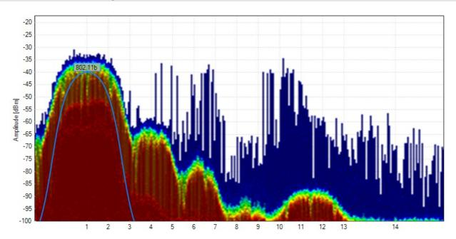
As 802.11b becomes less popular, this signature becomes less common, but it's good to be familiar with it. This **curve shape with lobes down each side** is made by an **802.11b** network, or any 802.11n network running at legacy data rates like 1, 5.5, or 11 mbps. Even an 802.11g or 802.11n network will fall back to this shape from time to time, or when idling. To prevent this, legacy data rates can be disabled, which will improve network performance.
