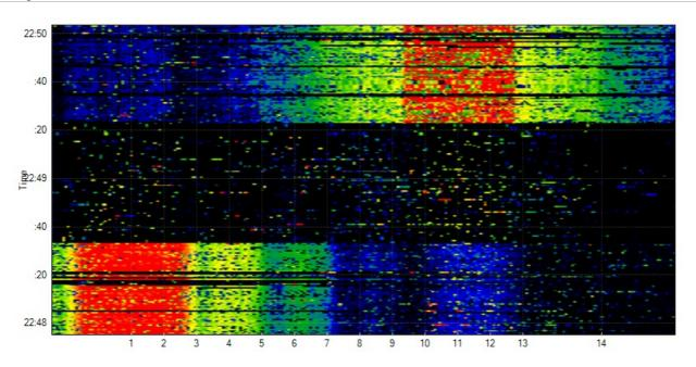
The Waterfall View graphs amplitude over time for each frequency in the band, much like a seismometer graphs earthquakes over time. The colors represent power levels in the spectrum with dark blue as low and bright red as higher amplitude levels - much like a
