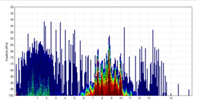
The **Overview Pane** shows you what is currently happening in the spectrum around you.. With **Color by Utilization** enabled, the intensity of the color shows how often a signal occurs. The more intense the color, the more often the spectrum is in use. This is called utilization, duty cycle, or air time usage.
