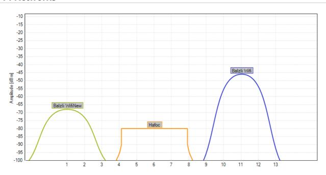
Both of your networks are on Wi-Fi channels 1 and 11. While there are two networks on channel 6, they aren't very close by. You could move your network on channel 11 to channel 6, which would give your ZigBee devices their very own channel to live on.
