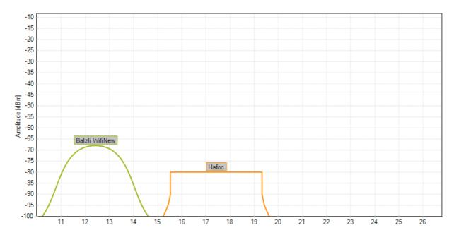
With Balzli Wi-Fi moved to channel 6, ZigBee channels 21-26 would be available for use with no competition from Wi-Fi networks
