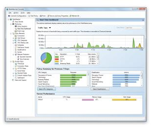
Trustwave webmarshal's real-time dashboard presents a range of information and useful statistics in a clear, easy-to-use interface. Recent web traffic by protocol is shown here including http, https, ftp, streaming media and instant messaging.
