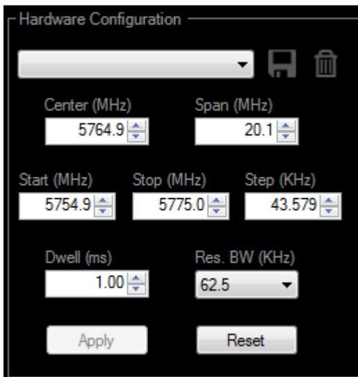
There are two methods in manually selecting the frequency range for the Wi-Spy configuration. You can enter a center frequency and select the frequency span or step width. For example, if you entered 5775 into the Center Field and 20 for the span it would leave 10 MHz on both sides of the center frequency. Alternatively, you can enter the start and stop frequencies. The Step Size and the Span are configured to automatically display at least 10 data points.
