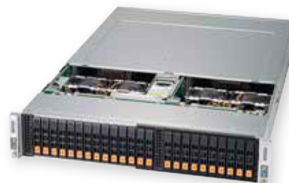
2U, 2 nodes BigTwin with 24 NVMe SSDs or 12 NVMe SSDs per node
